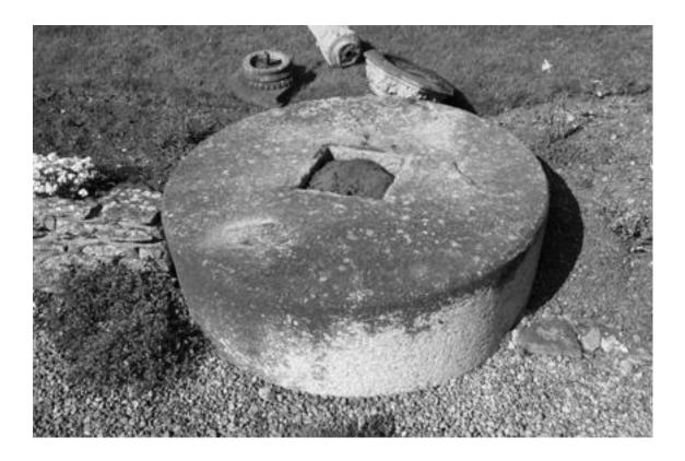
On inspection it was clear that this was some type of milling stone, but as it had no grooves in the main surface it is also clear that it was not a mill stone as used for flour etc. Its depth (around 450mm) is about twice the typical depth of such stones. Its diameter is around 1200mm and the square spindle hole about 300mm across. It was apparently cut from granite or another similar very hard stone, with flecks of mica visible.
